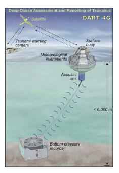
The DART 4G system consists of a surface buoy tethered to an anchored seafloor bottom pressure recorder (BPR)
